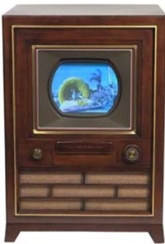
The CT-100 model color television had a viewing screen measuring about 9 x 11 inches.
